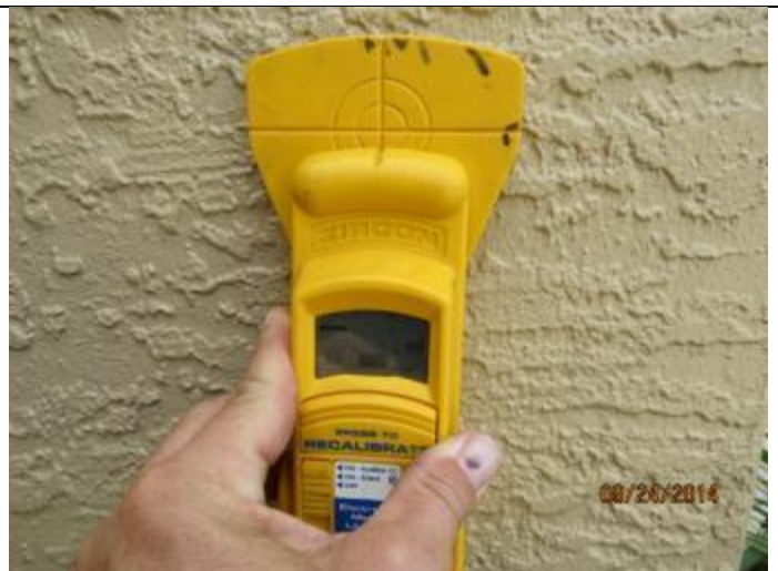
PHOTO 14 – Exterior Walls = Reinforced Masonry
