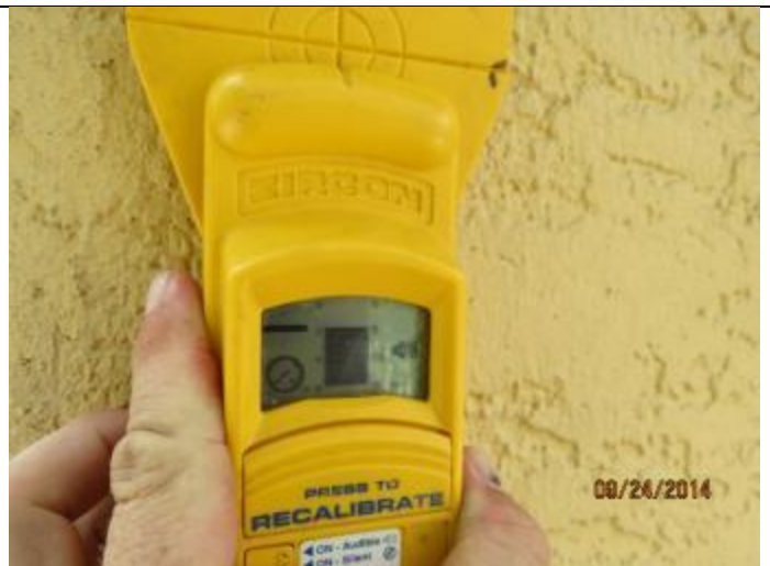
PHOTO 14 – Exterior Walls = Reinforced Masonry
