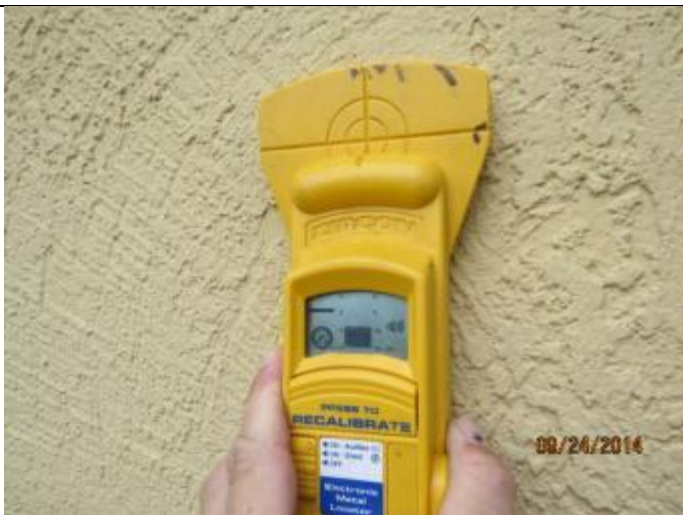
PHOTO 13 – Exterior Walls = Reinforced Masonry
